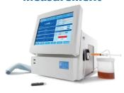
This property is tested on a Rudolph DDM series density meter. This instrument is a very simple to use. It is self-contained, there is no glassware or balance needed. Just inject the sample and get the result.
