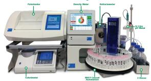
For smaller cleaning product companies just getting into testing, the 3 stand-alone instruments shown above will be enough to check incoming quality and allow a company to be certified according to ISO etc. When the sample volume is higher though and skilled staff are in short supply the package can be automated to measure Refractive index, optical rotation, specific gravity, color and pH all in one operation.
